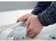
PLACE ON TRUCK WITH PRINT FACING YOU, APPLY PRESSURE TIP\* CHECK BEARINGS ARE IN SECURELY BEFORE MOVING ON TO NEXT STEP
