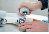
REMOVE BEARING, ROTATE WHEEL AS YOU PUSH TO HELP REMOVE
