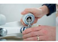
REMOVE BEARING, ROTATE WHEEL AS YOU PUSH TO HELP REMOVE
