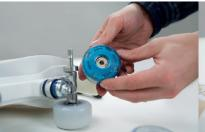
ONCE FIRST BEARING IS IN PLACE, ADD MAGNETIC TRIGGER FROM BOTTOM
